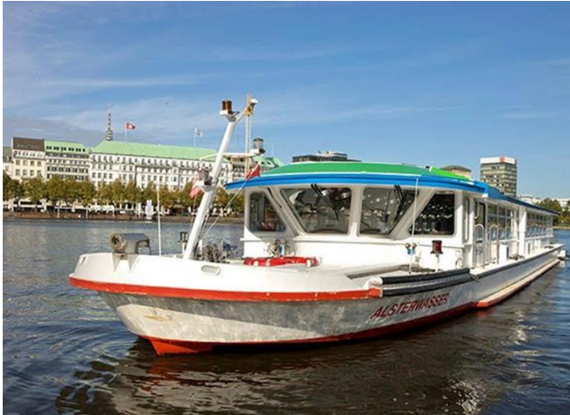
Zemship , 96 kW PEMFC with battery
