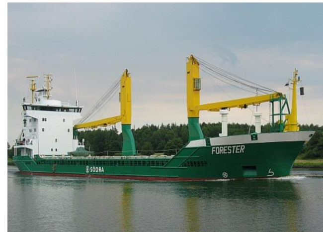
Forester , 2009-2017 (phase1), 2017-2022 (phase2) 100 kW SOFC with DE and battery
