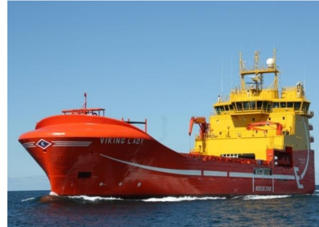
Viking Lady , 320 kW MCFC with DE and battery
