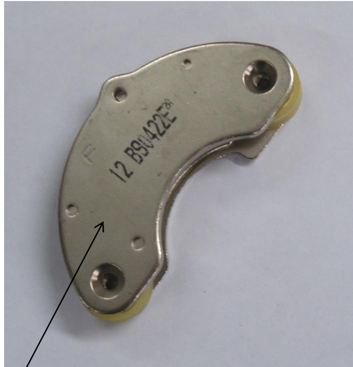
Voice coil assembly extracted from hard drive
