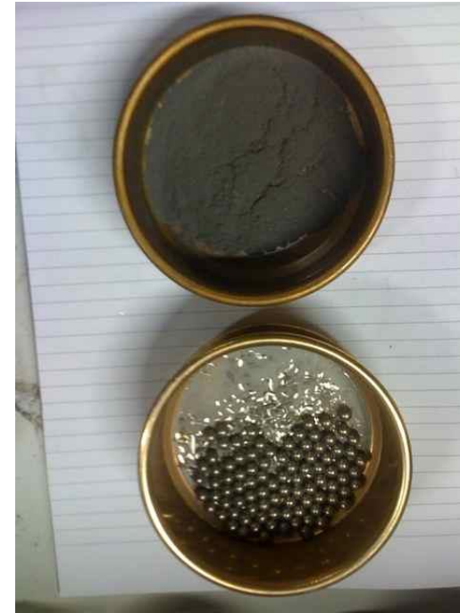
Sieving with ball bearings has been used to preferentially break down the NdFeB compared to the Ni and other impurities
