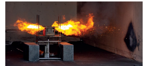
93Ah NMC prismatic cell hard venting against representative battery enclosure lined with AIS' thermal barrier material
