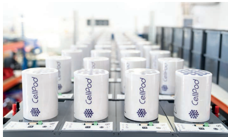
CellPod One: individual thermal chambers, which are surface cooled and independently thermally controlled
