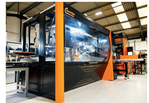
Electrified Automation's fully automated stator assembly
